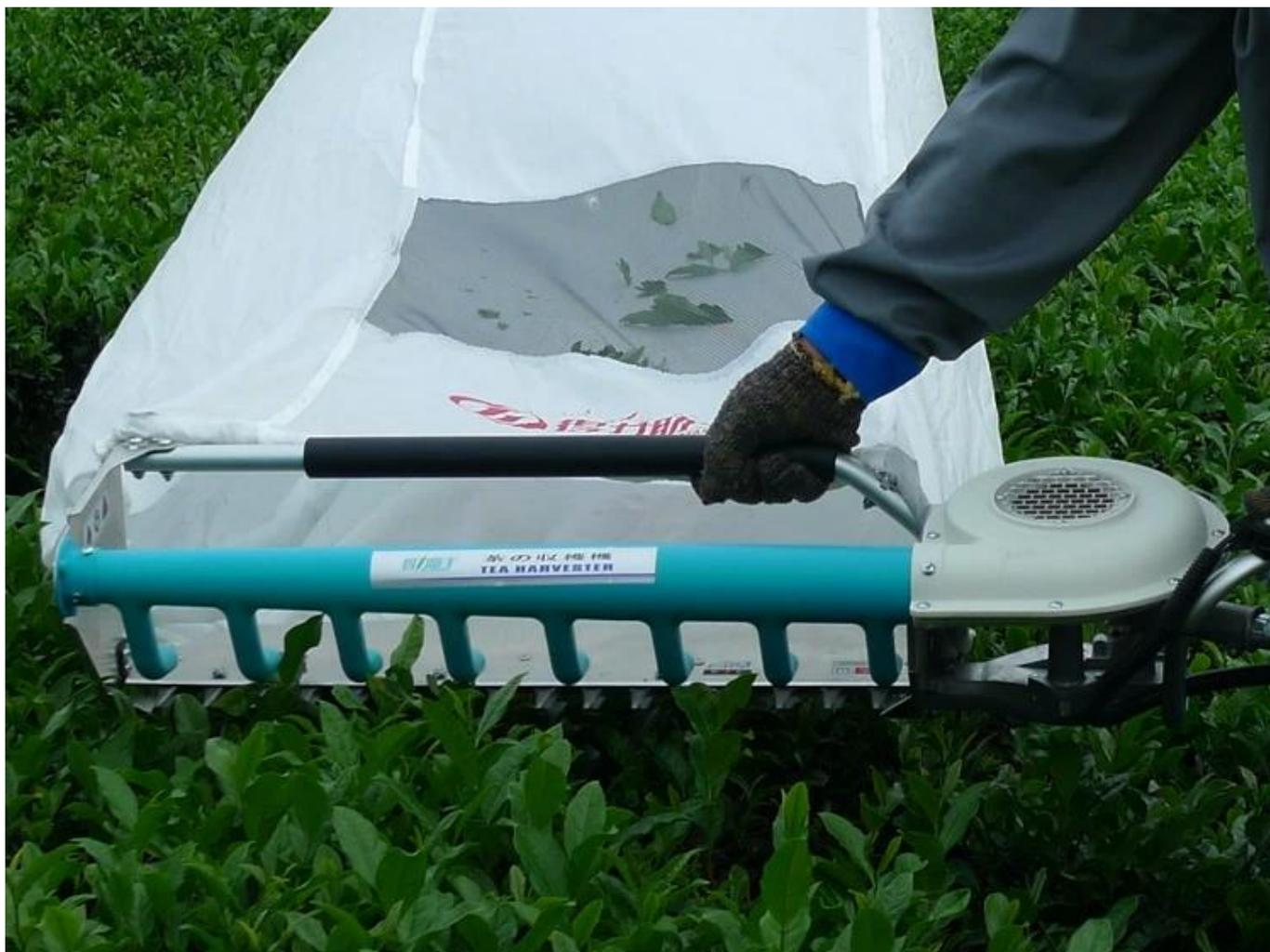
Gasoline Tea Harvester Machine is a manual machine used for harvesting tea leaves. It is designed to be used in tea plantations and is suitable for harvesting tea leaves in a large area. The machine is easy to operate and can be used by a single person. It is a good choice for tea growers who want to increase their harvest efficiency and reduce labor costs.
