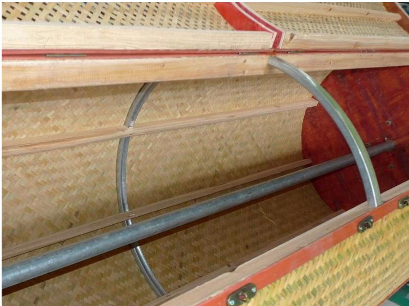
Figure 1 shows the internal structure of the boat, which is made of wood and woven bamboo. The boat is painted red on the outside. The internal structure is made of wooden planks and metal rods. The woven bamboo walls are visible on the left and right sides. The metal rods are visible in the center and bottom of the boat.
